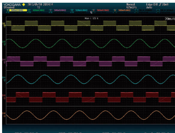
Power parameter measurement of three-phase motor
